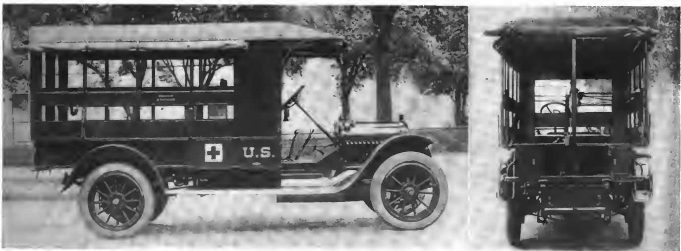
Above is one of the new U. S. army standard ambulances, this particular vehicle being one of fifty-two recently built by the White Co., Cleveland, for service on the Mexican border. These machines have been organized into four companies, each composed of twelve motor ambulances and one \frac{3}{4} -ton repair truck. The plan of organization and the new body designs were worked out by a board consisting of Major Robert E. Noble, Major A. W. Williams, Major P. L. Jones and Captain A. C. Christie. The design has a capacity for eight patients seated inside and an orderly riding on front with the driver. Four patients can be carried on stretchers or litters. The two litters composing the upper tier are suspended by iron hooks with spiral spring attachments. The seats are leafed and hinged in such a manner that when they are not occupied by sitting patients the upholstered side is turned down, forming a floor on which standard U. S. Army litters may be carried. Under these deck-seats are compartments for ten 1-gal. tins of reserve gasoline and other supplies. Beneath the front seat on each side are compartments for carrying water tanks. Between the stanchions at the right of the driver's seat is a compartment for carrying emergency medicines and dressings.
